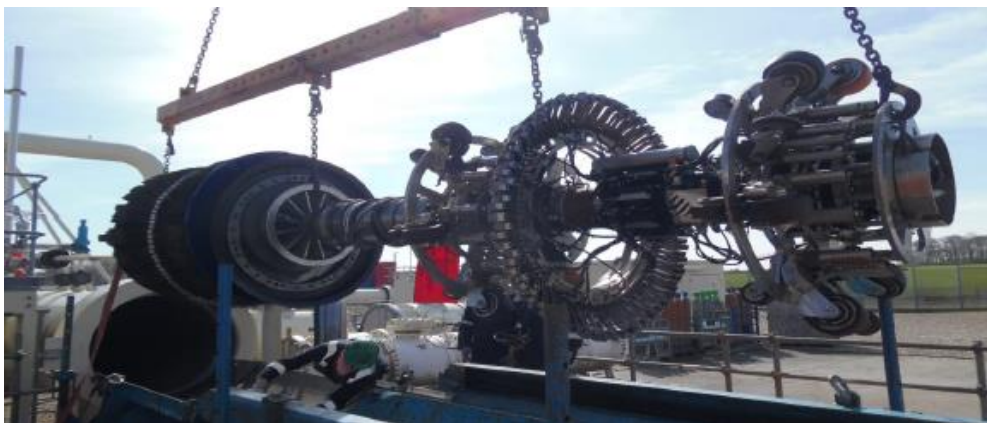
Image 3 = Main Inspection Gauge
