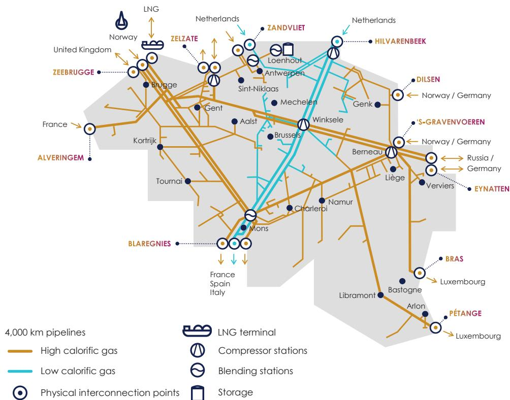
In Belgium, the company owns and operates 4,000 km of natural gas transmission pipelines and associated infrastructure as well as the underground storage facility in Loenhout, where natural gas is stored in aquifers more than one kilometre under the ground. Fluxys LNG (a wholly owned subsidiary of Fluxys Belgium) owns and operates the terminal for liquefied natural gas (LNG) in Zeebrugge.
