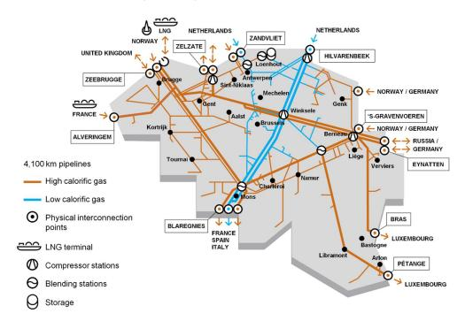
The Fluxys Belgium transmission grid in Belgium has about 4,100 kilometres of pipelines and several physical connections, opening up the Belgian grid to natural gas flows from the United Kingdom, Norway, the Netherlands, Russia and all LNG producing countries. The Fluxys Belgium grid also serves as the crossroads for natural gas transmission flows to the Netherlands, Germany, Luxembourg, France, the United Kingdom and Southern Europe.
