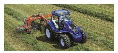
New Holland methane-powered tractor
