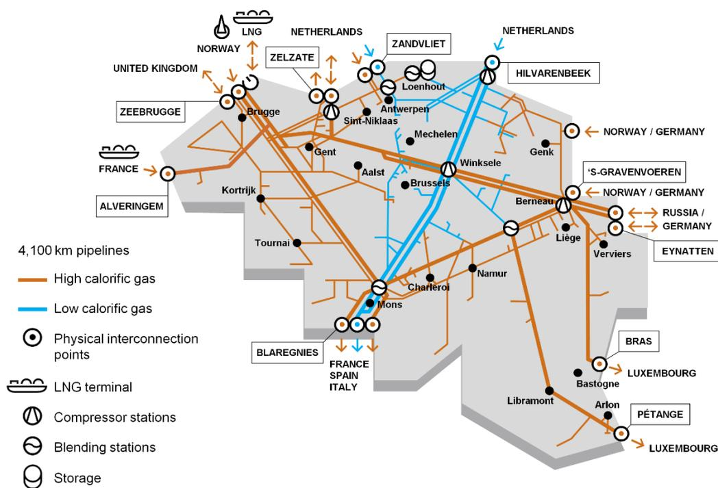
The Fluxys Belgium transmission grid in Belgium has about 4,100 kilometres of pipelines and several physical connections, opening up the Belgian grid to natural gas flows from the United Kingdom, Norway, the Netherlands, Russia and all LNG producing countries. The Fluxys Belgium grid also serves as the crossroads for natural gas transmission flows to the Netherlands, Germany, Luxembourg, France, the United Kingdom and Southern Europe.
