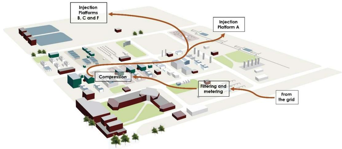
**Filtration and metering.** Incoming natural gas is first filtered in order to prevent the dust it contains from damaging the facilities. The filtered gas then passes through a metering line which measures its volume, pressure and temperature. The composition of the gas is also analysed. All the data are forwarded to the on-site control room for further processing.
