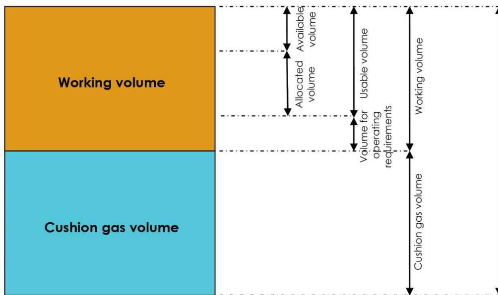
Taking into account the operating conditions at the storage facility, Fluxys Belgium determines the **working volume** in order to establish both the flow rates and withdrawal conditions (including pressure) which are feasible and compatible according to the geological characteristics of the reservoir.
