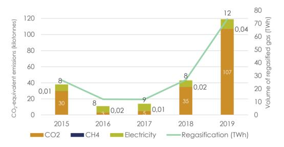
LNG terminalling: greenhouse gas emissions
