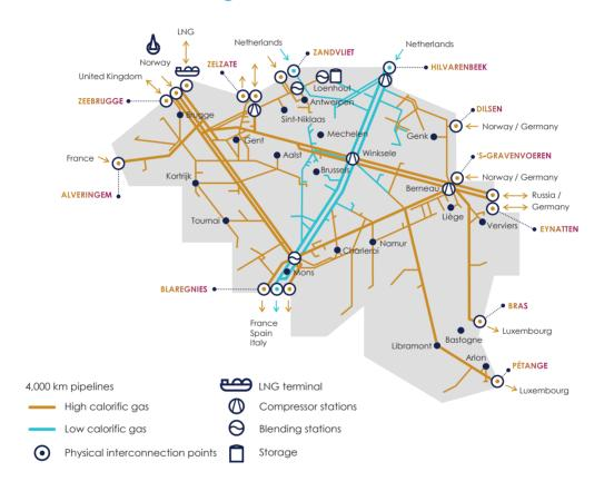
In Belgium, the company owns and operates 4,000 km of natural gas transmission pipelines and associated infrastructure as well as the underground storage facility in Loenhout, where natural gas is stored in aquifers more than one kilometre under the ground. Fluxys LNG (a wholly owned subsidiary of Fluxys Belgium) owns and operates the terminal for liquefied natural gas (LNG) in Zeebrugge.
