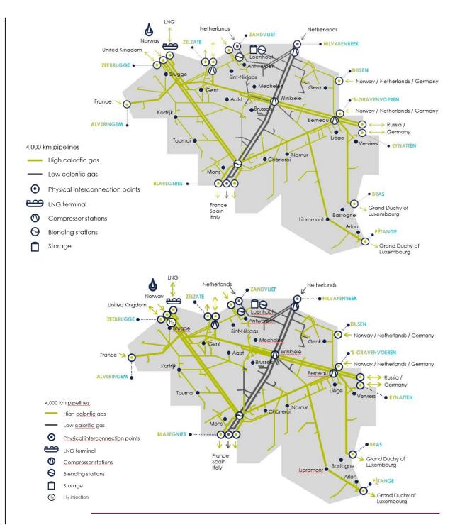
The Fluxys Belgium transmission grid in Belgium has about 4,000 kilometres of pipelines and several physical connections, opening up the Belgian grid to natural gas flows from the United Kingdom, Norway, the Netherlands, Russia and all LNG producing countries. The Fluxys Belgium grid also serves as the crossroads for natural gas transmission flows to the Netherlands, Germany, Luxembourg, France, the United Kingdom and Southern Europe.
