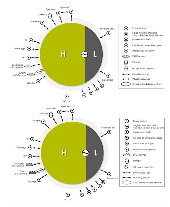
An interconnection point is a type of connection point<sup>3</sup> linking the Fluxys Belgium transmission grid with the transmission grid of an adjacent TSO.
