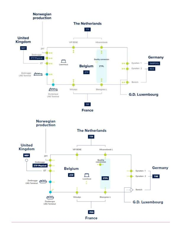
According to EU Commission Regulation 2017/459 (CAM NC), transmission system operators shall offer the available capacities at different Interconnection Points connecting the same two Entry/Exit systems at a Virtual Interconnection Point (VIP).
