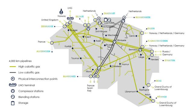
The Fluxys Belgium transmission grid in Belgium has about 4,000 kilometres of pipelines and several physical connections, opening up the Belgian grid to natural gas flows from the United Kingdom, Norway, the Netherlands, Russia and all LNG producing countries. The Fluxys Belgium grid also serves as the crossroads for natural gas transmission flows to the Netherlands, Germany, Luxembourg, France, the United Kingdom and Southern Europe.
