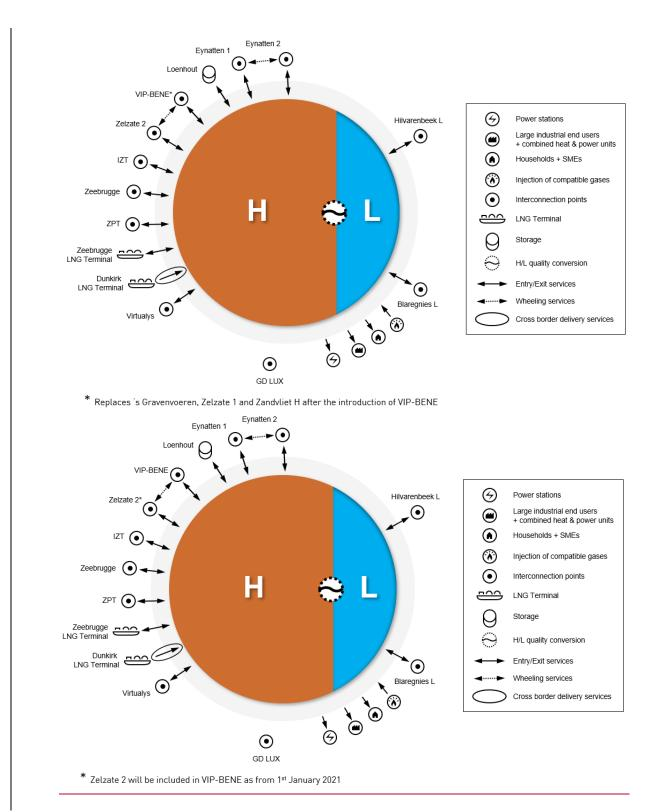
An *interconnection point* is a type of connection point<sup>3</sup> linking the Fluxys Belgium transmission grid with the transmission grid of an adjacent TSO.
