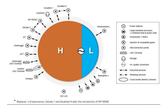
An interconnection point is a type of connection point<sup>3</sup> linking the Fluxys Belgium transmission grid with the transmission grid of an adjacent TSO.
