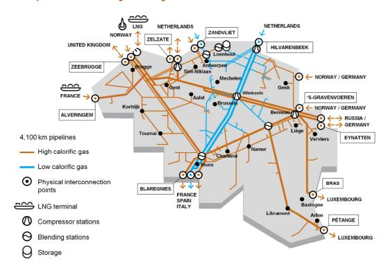
The Fluxys Belgium transmission grid in Belgium has about 4,100 kilometres of pipelines and numerous several physical connections, opening up the Belgian grid to natural gas flows from the United Kingdom, Norway, the Netherlands, Russia and all LNG producing countries. The Fluxys Belgium grid also serves as the crossroads for natural gas transmission flows to the Netherlands, Germany, Luxembourg, France, the United Kingdom and Southern Europe.
