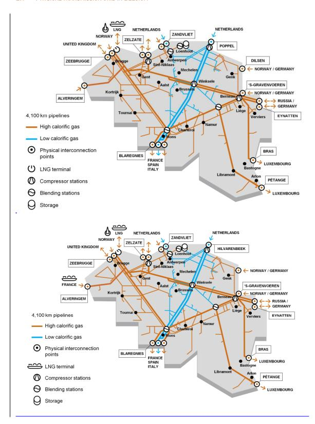
The Fluxys Belgium transmission grid in Belgium has about 4,100 kilometres of pipelines and 20 interconnection points, opening the Belgian grid to natural gas flows from the United Kingdom, Norway, the Netherlands, Russia and all LNG producing countries. The Fluxys Belgium grid also
