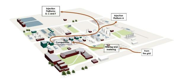
**Filtration and metering.** Incoming natural gas is first filtered in order to prevent the dust it contains from damaging the facilities. The filtered gas then passes through a metering line which measures its volume, pressure and temperature. The composition of the gas is also analysed. All the data are forwarded to the on-site control room for further processing.
