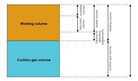
Taking into account the operating conditions at the storage facility, Fluxys Belgium determines the **working volume** in order to establish both the flow rates and withdrawal conditions (including pressure) which are feasible and compatible according to the geological characteristics of the reservoir.
