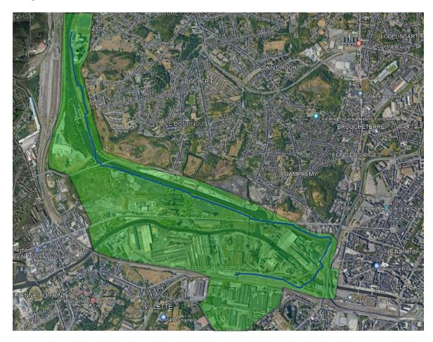
The above described pipeline routing must be seen as indicative, but gives a clear overview of the most probable H<sub>2</sub> network development in the area of Charleroi, and therefore the highest likelihood to have an easy access to the network from within the proposed coverage area (coloured).
