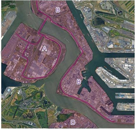
The above described pipeline routing gives a clear overview of the most probable CO<sub>2</sub> network development in the port of Antwerp region, and therefore the highest likelihood to have an easy access to the network from within the proposed coverage area (coloured).
